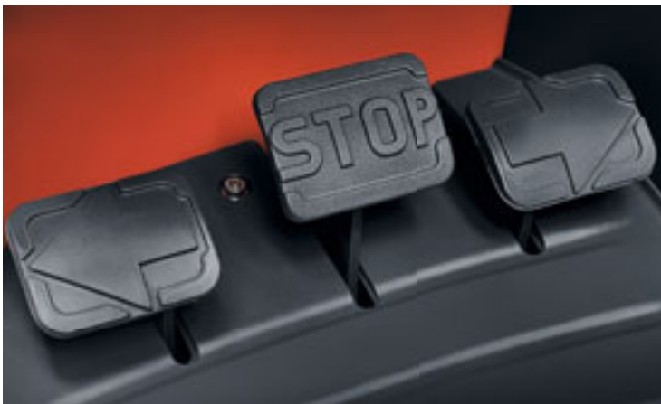
Linde twin accelerator pedal format – seamless reversing without switching feet
