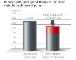
**Tests show** that low revolution speeds reduce fuel consumption, emissions and wear.
