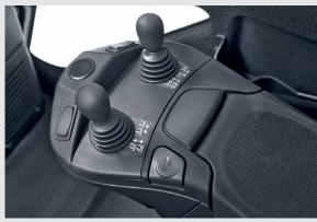
**Linde Load Control**. Even gentle hand movements are enough to position heavy loads precisely and safely.
