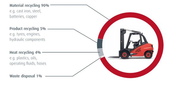
Even at the end of their long service life, Linde trucks continue to impress. As Linde uses a production process that consistently employs homogeneous and reusable materials, its trucks are 99% recyclable.
