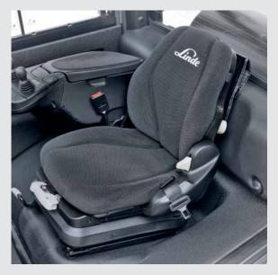
In addition to an abrasion-resistant fabric covering, the **comfortable seat** coated with activated carbon provides mechanical lumbar support and optional air suspension.
