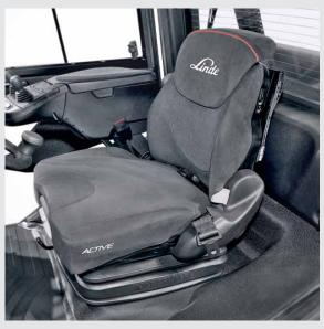
High-end comfort for long periods of use. The "super comfort **active**" with ergonomic seat and backrest and a world first in truck manufacture: climate control equipment with active ventilation.
