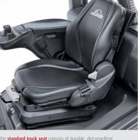
The **standard truck seat** consists of durable, dirt-repellent PVC. The mechanical spring assembly offers 60 mm of spring travel for drivers weighing up to 130 kg.
