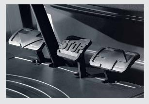
Forward and reverse travel with no need to change over feet, thanks to **Linde dual-pedal control**.
