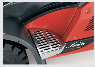
The stable, **stainless steel step** ensures drivers can get in and out of the truck safely.
