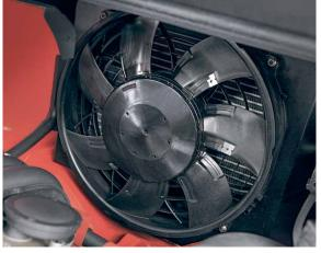
**Sophistication in every last detail**. The newly developed electric fan adapts its speed to the temperature of the hydraulic oil, coolant and charge air, making it significantly more economical.
