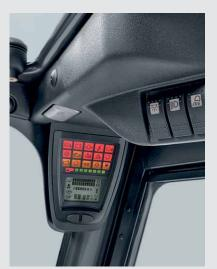
The **display** is fitted in the upper part of the cockpit, meaning it is always in the driver's field of vision. The illuminated symbols are easy to see.
